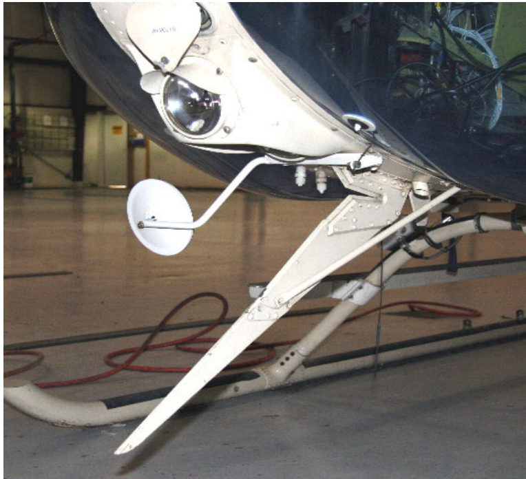
Examples of items prohibiting the installation of the G1 and Cineflex on Bell 206 and 407 series
