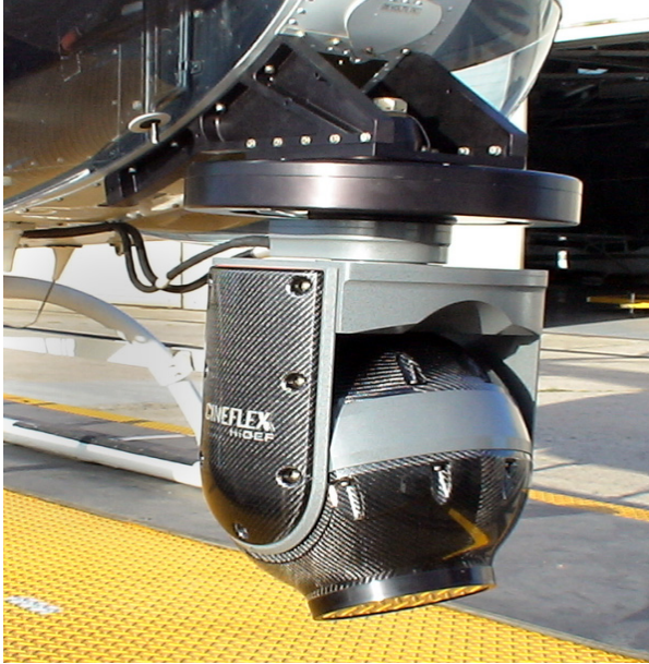
G1-1 Nose Mount with Vibration Isolator and Cineflex V14 Gimbal
