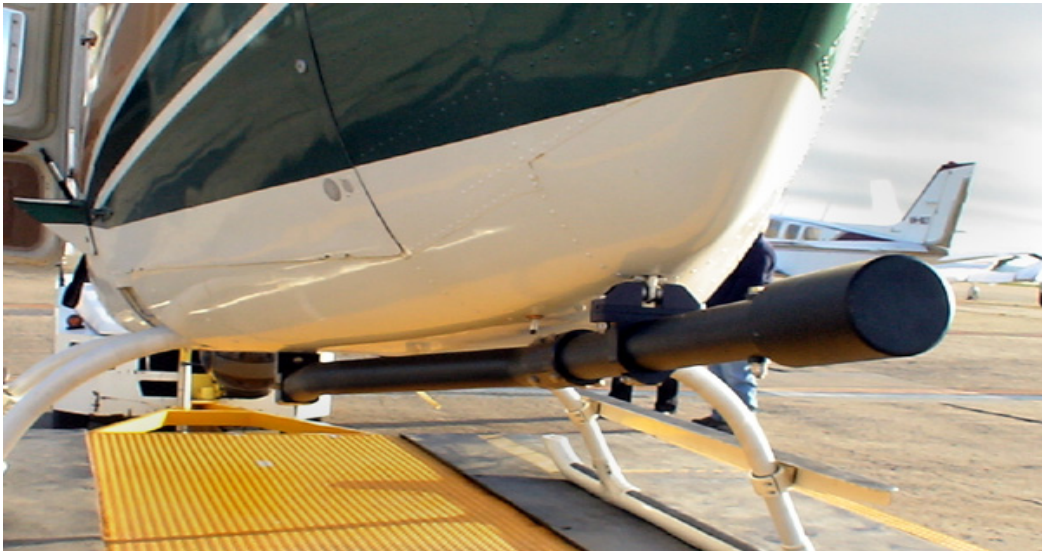
G2-1 Counterweight Assembly installed on Bell 206
