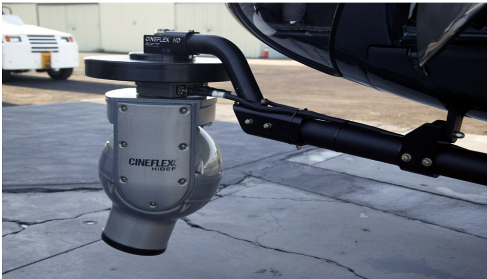
AFSP-1 with Vibration Isolator mounted on AS350 B3
